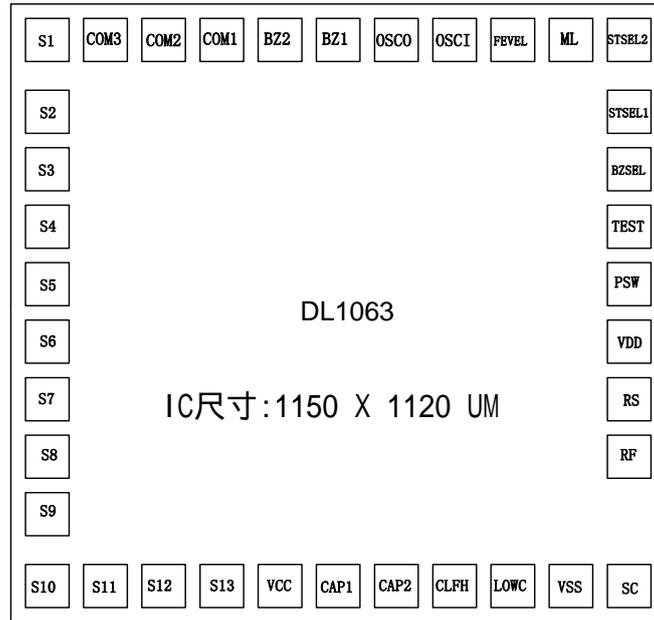
Note: The IC substrate should be connect to VSS
